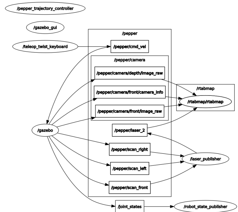
FIGURE 3.14: RQT graph with Gazebo, Pepper and RTABMAP nodes and topics
